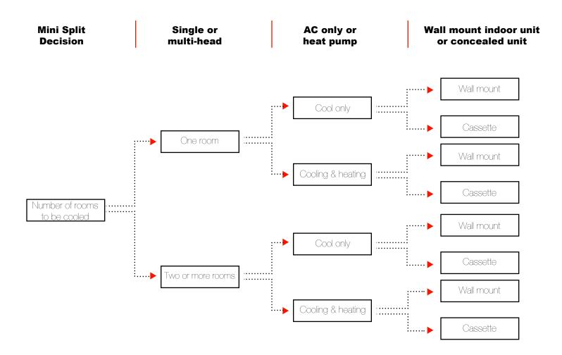
A single head has one indoor unit matched to an outdoor unit. A multi head combines an outdoor unit with a unit that has a max of 5 indoor units. The indoor unit can be different sizes, in different rooms.
